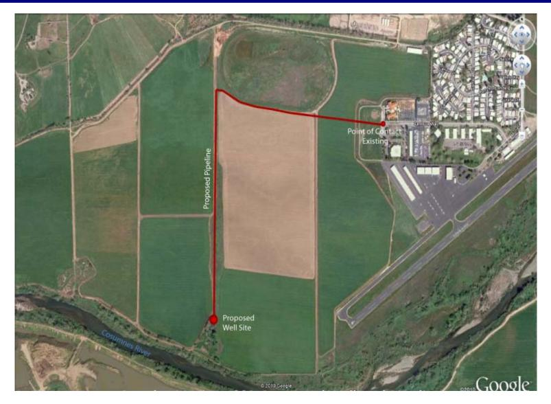
Figure 28: Rancho Murieta CSD Proposed Well and Pipeline
