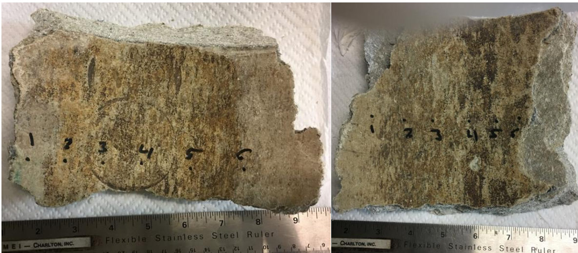
Figure 2b: Inside view of the pipe section wall of Sample 1 (left) and Sample 2 (right)
