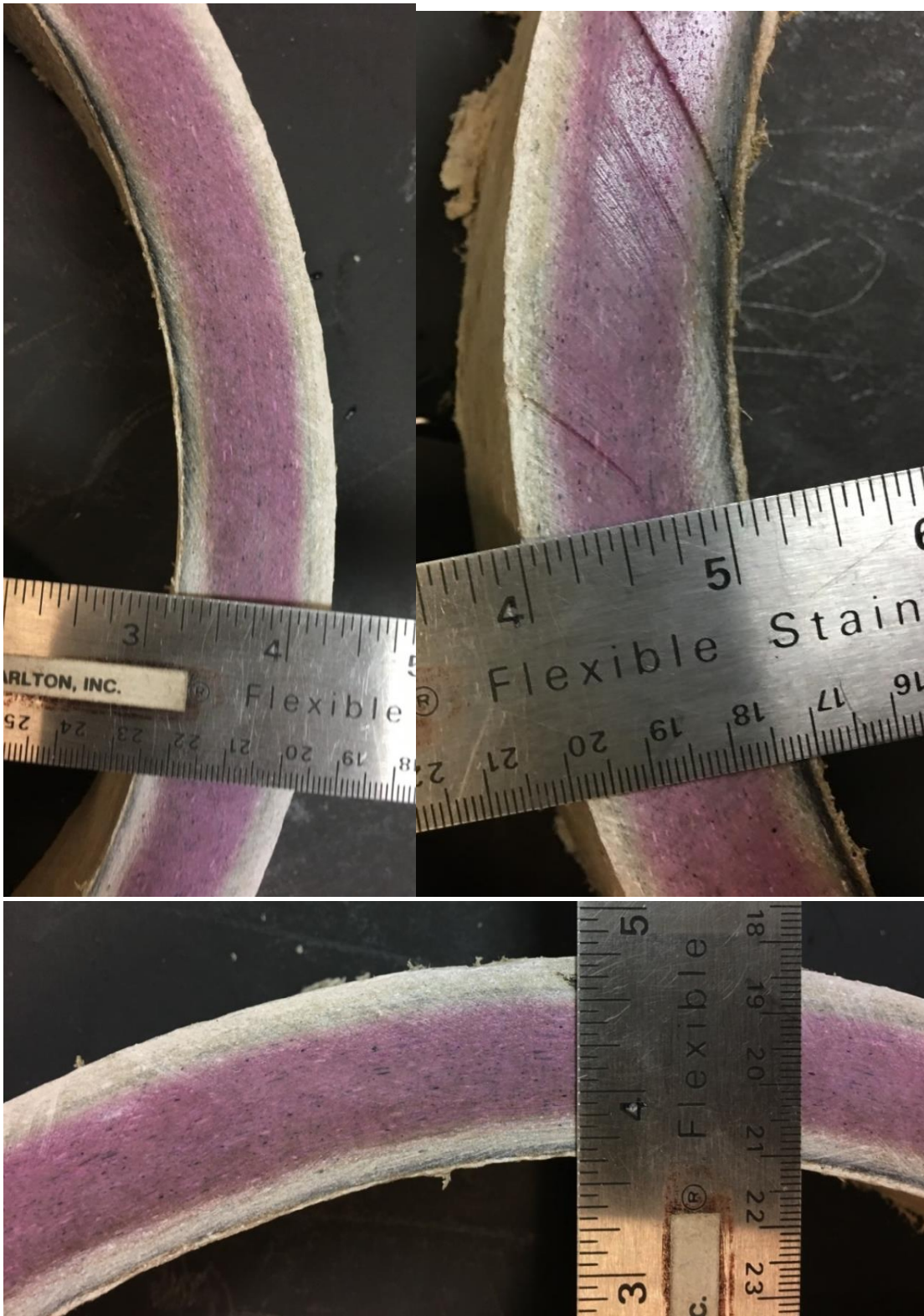
Figure 8: Photograph of Sample 3 wall cross section showing maximum attack depth locations
