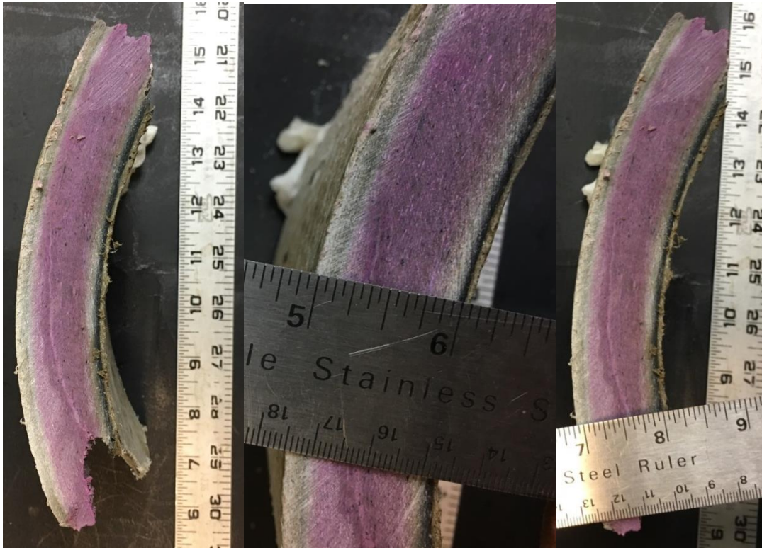
Figure 6: Photographs Sample 2 wall cross section after staining with phenolphthalein. Note the white areas showing loss of alkalinity
