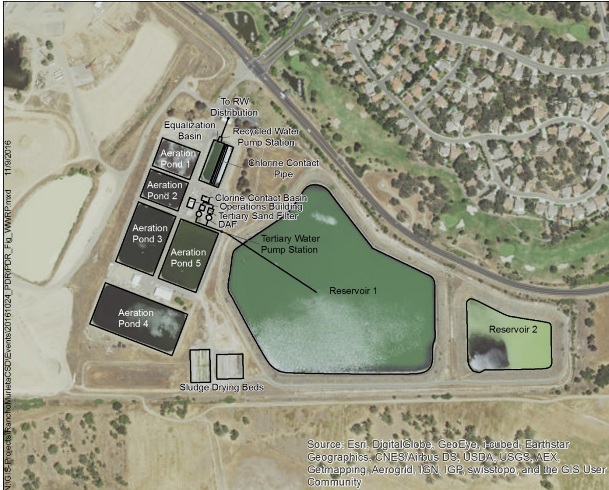
Figure 10. Existing WWTF and WWRP
