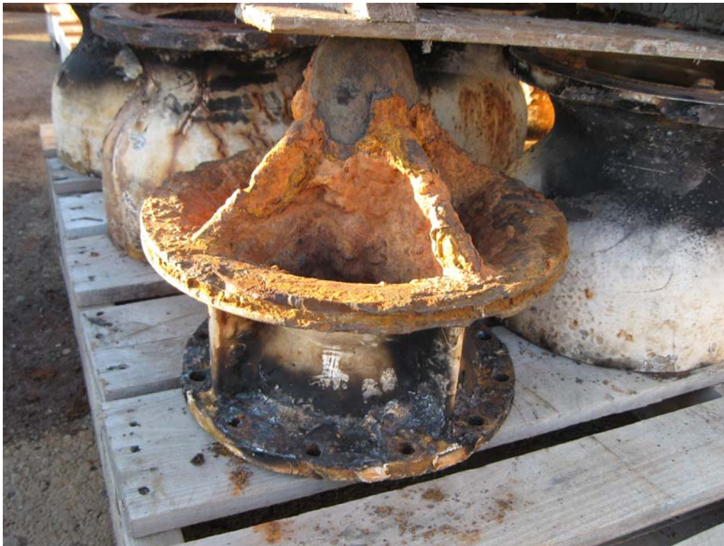
Figure 1 - Suction bell center bearing support cracked due to shaft whipping
