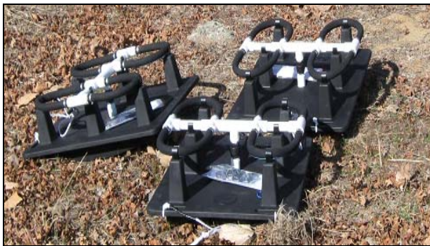
Aeration pods which will sit at bottom of basin
