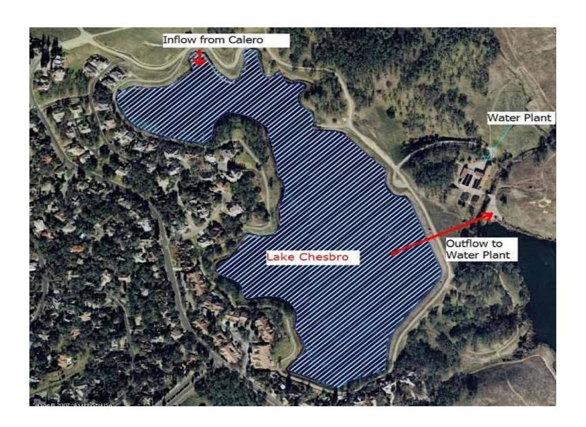
Aeration in lake Chesbro is used to keep the lake mixed & oxidize Iron or Manganese
