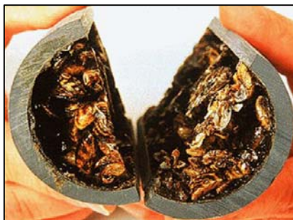
Pipe cross-section inundated with invasive Mussels
